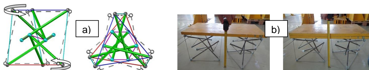
Fig. 2 a) A structure built on the Class \Theta=1 triangular tensegrity prism as 3D example of an auxetic metamaterial, that is material with a negative Poisson’s ratio. b) After loading both prismatic modules by one steel plate with mass 28 [kg], the initial height did not change noticeably. After a two-fold increase in the load (two plates with a total mass of 56 [kg]), the initial height was reduced by 4 [mm]. The mass of one prismatic module made of steel is less than 1.5 [kg].
